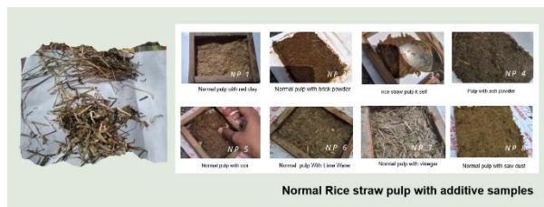
Figure 3: Normal Rice straw-based pulp composite samples – Compressive Strength and Water absorption
