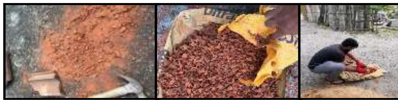
Figure 4 : Photographs of the alternative coarse aggregates produced
