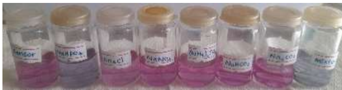
Figure 6-: (a) The solution series of the sensor with different concentrations of ions. From left to right: Sensor, \text{HPO}_4^- , \text{Cl}^- , \text{NO}_2^- , \text{SO}_4^{2-} , \text{HCO}_3^- , \text{CO}_3^{2-} , and a mixture of ions
