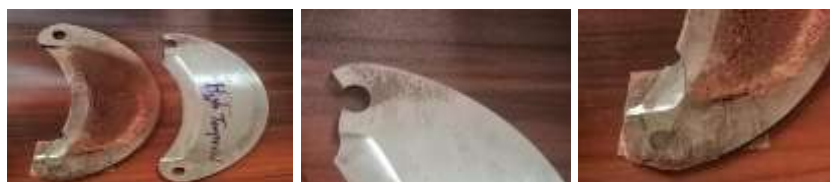
Figure 01. Fractured Type 01 blades during the chipping process
