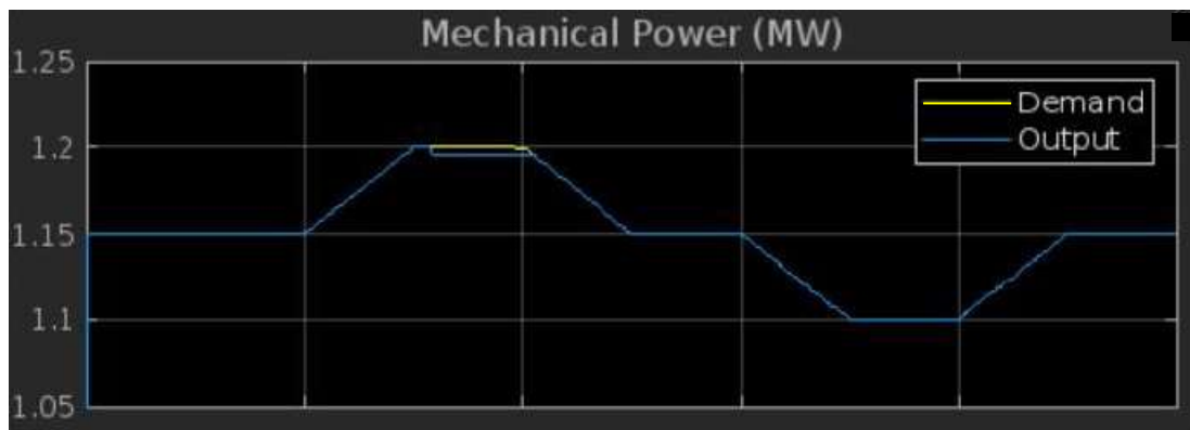
Figure 03: Mechanical Power Output of the Generator Vs Plant Load during the Islanded Operation
