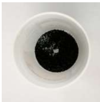
Figure 2. Synthesized iron nanoparticles in powder
