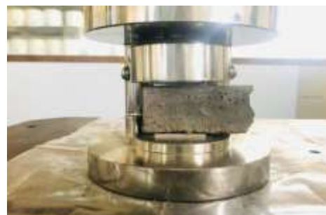
Figure 4. Compressive strength test
