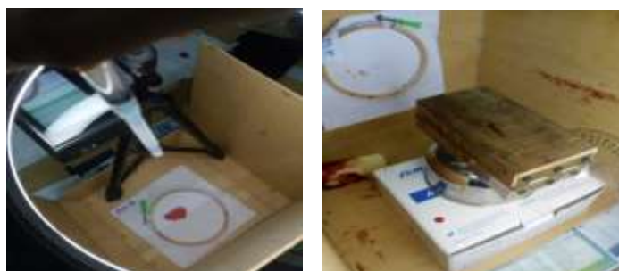
Figure 1: Drip tower apparatus (left) and modified mouse-trap apparatus (right)
