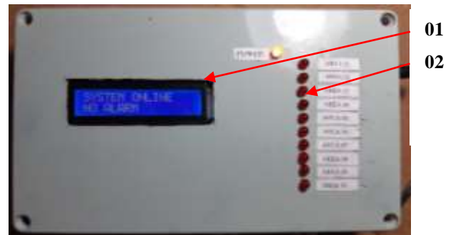
Figure 02: Fire control unit's system
