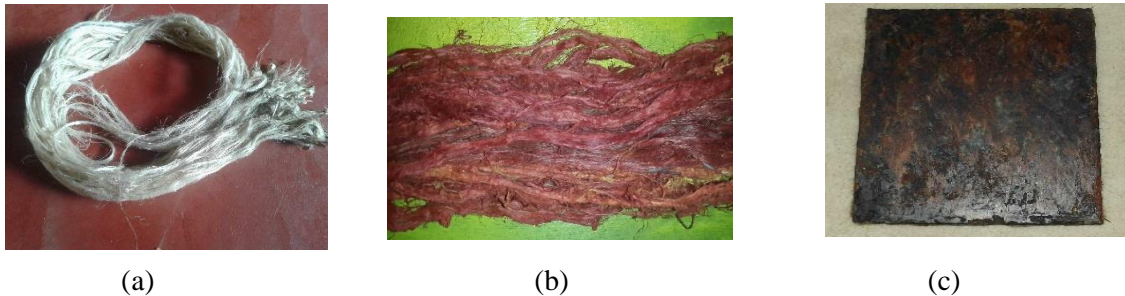
Figure 1: (a) Treated and dried PALF (b) Dyed PALF (c) PALF reinforced composite
