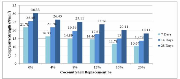
Figure 2: The relationship between Concrete Compressive Strength and Curing Days.
