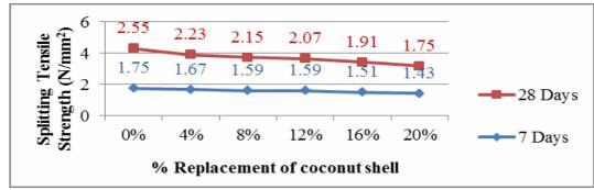
Figure 3: The relationship between Spitting Tensile Strength and a % Replacement of Coconut Shells
