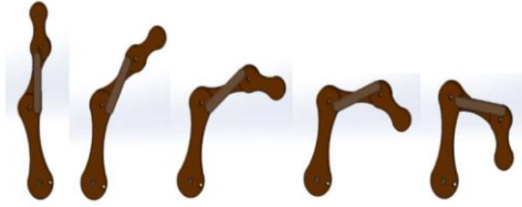
Figure 8. CAD Design and simulation of Finger movements
