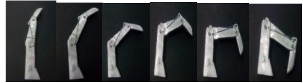
Figure 9. Implemented finger and its PP & DP joint movements
